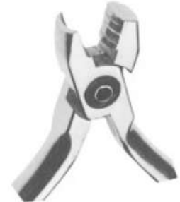
709-395-130 De La Rosa Arch Forming Plier 13 cm, 5" grooved. Designed to form and contour arch wires with or without torquing on round or rectangular wire. The beak has grooves of 0.41mm, 0.46mm, 0.56mm
