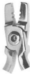
709-365-130 Lingual Arch Plier 13 cm, 5" used to form double and triple back bends in 0.76 or 0.91 wire for insertion in lingual sheaths.
