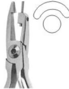
709-380-130 Single Diameter Loop Farming Plier. 13 cm, 5" The replaceable cylindrical back has only one diameter section of 1.52mm.
