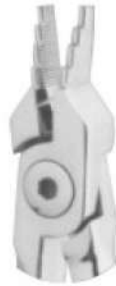
709-503-130 Loop Forming & Closing Plier 13 cm, 5" Precision loop forming with four step tip (3,4,5 & 6mm). Excellent for wires up to .022". Beveled edges prevent wire scoring & one serrated beak prevents wire slippage.
