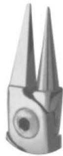
709-482-130 Light Wire Bending Plier 13 cm, 5" Designed for working on small wires and forming wire springs. Tapered beaks make it easy to bend small diameter loops. (Bends wires up to .020")
