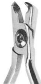
709-326-130 Distal End Cutter (non-holding). 13 cm, 5" A precision cutter designed for distal arch cutting. Cutting angle of 72 degree allows cutting of wire very close to distal end of buccal tube. Caution: maximum cutting capacity arch wire up to 0.56x0.71 mm rectangular, round wires up to 0.51 mm.
