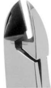
709-308-130 Oblique Pin & Ligature Cutter 13 cm, 5" By setting the cutting head at a 15 angle to the handles, you get better, more visible access to the working area. More professionals prefer oblique angled pin and Ligature cutters for wires up to .020".
