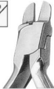
709-246-130 Tweed Arch Bending Plier 13 cm, 5" use this specialty plier to form offset and 90 bends on rectangular and square wires up to .022" x .028". Radiuses on tip edges do not mar or fray wire during torquing.
