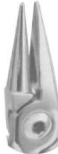
709-491-130 Occulist Plier 13 cm, 5" Round and concave beaks bend round or rectangular wire with a firm grip that will not nick wire. Bends wires up to .020".
